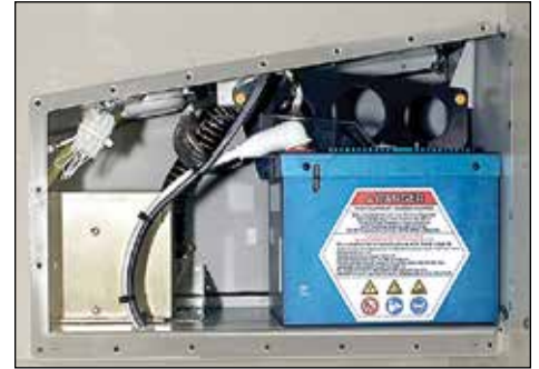
The TB17 Lithium-ion battery installed in an R66.
