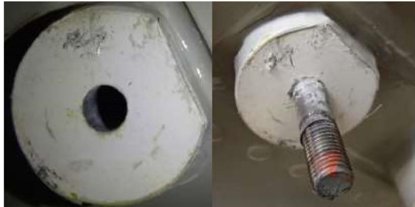
FWD upper attachment tail pylon with jammed bolt (r)
