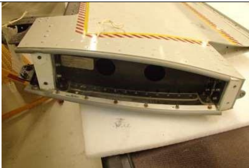
Overview horizontal stabilizer – attachment holes
