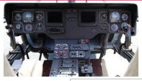
The basic cockpit of the Ansat – the aircraft can be flown with one or two pilots. (Photo: author)
