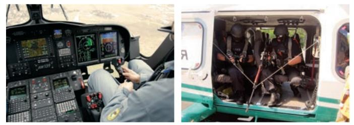
The AW139 was the first helicopter flown by SASU pilots to feature an advanced avionics outfit, including, among others, a sophisticated autopilot, large cockpit displays and dual FMS. The spacious cabin allows a police sniper team to provide fire support from the air.
