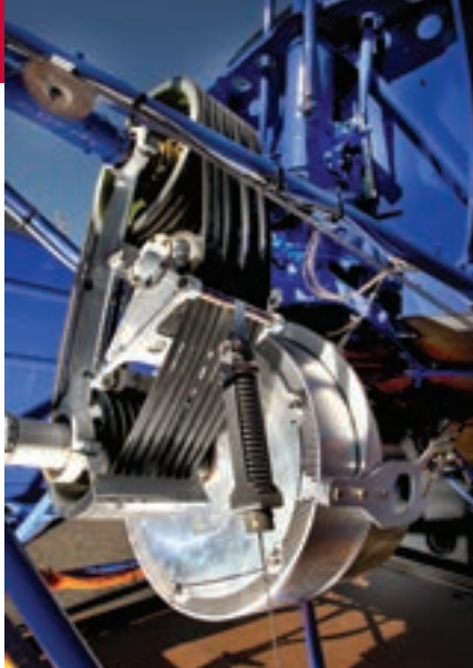
The US Hybrid electric motor on the Firefly is half the weight of the piston engine it replaces. (Photo: Sikorsky)
