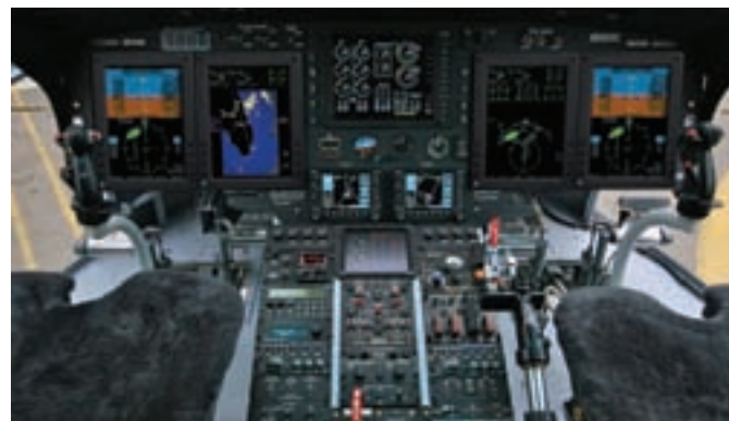
Under the ODICIS project, Thales has developed a single display that stretches across the cockpit (left), offering the same flight information as multiple-MFD suites like Rockwell Collins' Pro Line 21 (right). (Photos: Thales/Rockwell Collins)
