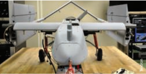
Shadow hardware-in-the-loop simulator at the Textron Systems and Bell/AAI research lab in Huntsville, Ala.
