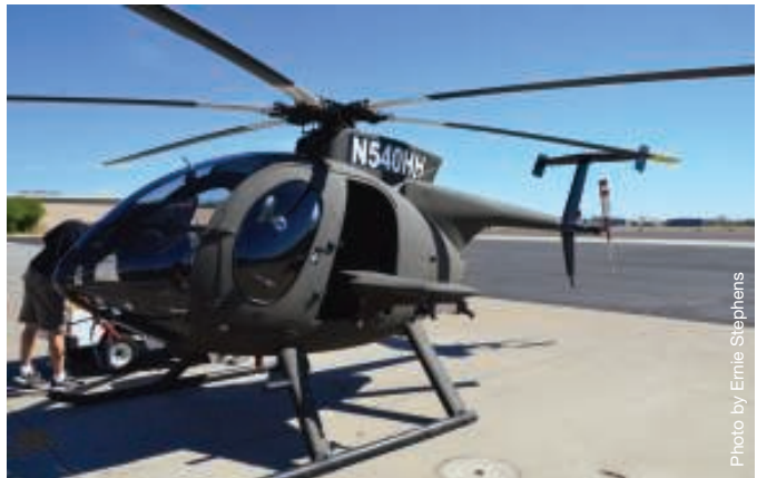
The MD540F can carry a variety of missiles and guns on each end of its weapons ring. The structure doubles as a 62.1-gallon auxiliary fuel tank.
