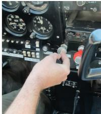
would move to the fully open position under the action of the bias spring. While there are different types of throttle control systems which are intended to prevent the throttle opening in similar circumstances, it is always important to check that the throttle, and its friction device, is set in the correct position for starting.
