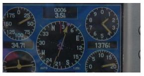
However, technology moves on. Many pilots keep a GPS set in their field of view. Several of these instruments can be set up before joining the pattern to give prominence to the aircraft's groundspeed. If, for example, the groundspeed displayed on the downwind leg is less than our indicated airspeed, that would warn of a likely tailwind on final and suggest an early and safe go-around.
