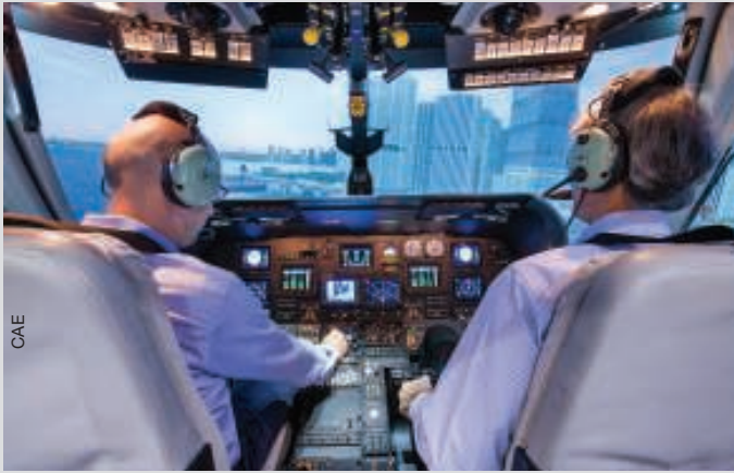
The 3000 series features a 210-degree horizontal by 80-degree vertical view for training.
