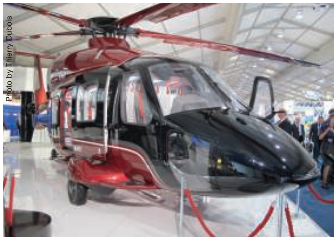
The Ka-62, a civil derivative of the military Ka-60, features new elements such as Turbomeca engines, a Transas avionics suite and a crashworthy fuel tank.
