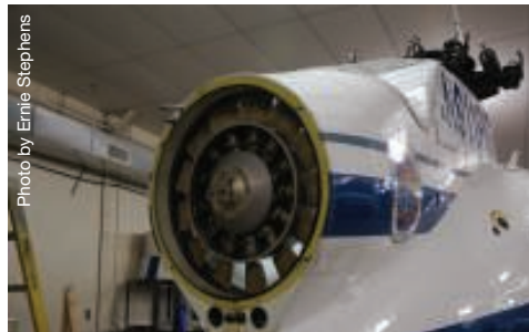
Photo by Ernie Stephens With the tail boom removed, the details of the NOTAR fan on this MD520N are easy to examine. The screened opening of its air intake can be seen behind the main rotor hub.
