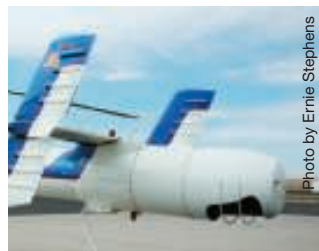
The rotating cone on this MD Explorer remains parked in this position until pedal inputs turn it to direct air in one direction or the other.
