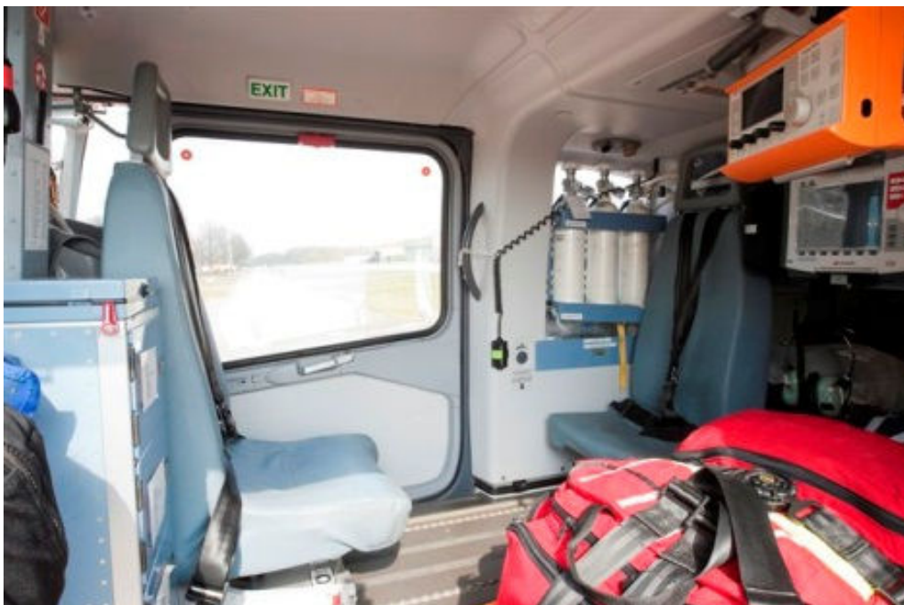
The medical interior with the doctor swivel seat (LH) and passenger/ medic seat (RH) and oxygen bottle's installed.
