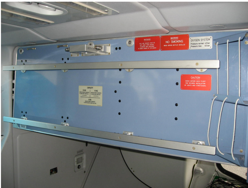
The medical wall (for installation of medical equipment)
