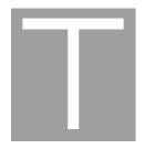
A white landing T signifies that aeroplanes and gliders taking-off or landing shall do so in a direction parallel with the shaft of the T and towards the cross arm, unless otherwise authorised by the appropriate ATC unit.
