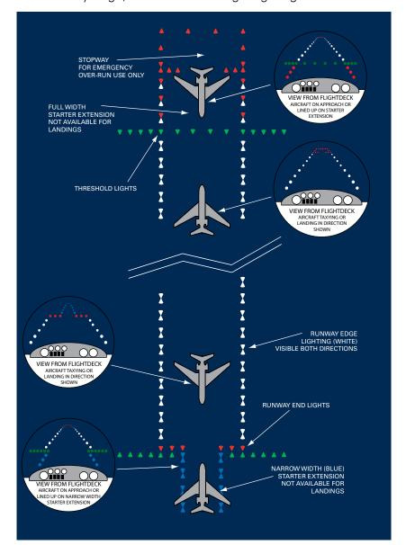
Figure 1.5 Runway Edge, Threshold and Edge Lighting
