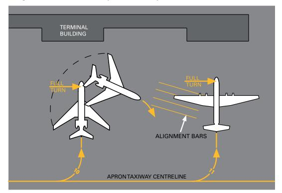
Figure 2.4 Self Manoeuvring Stand Markings
