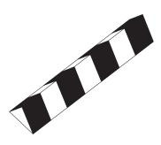
At displaced thresholds on both side of runway.
