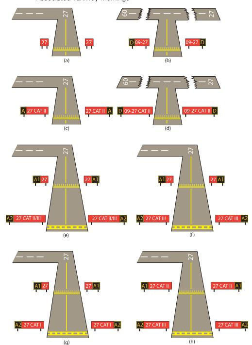
**Figure 3.2** Typical Runway Taxi-Holding Position Signs and Associated Taxiway Markings
