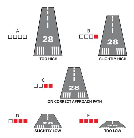
Where used together with ILS, PAPI is located so as to ensure, as far as is practicable, correlation between the two approach paths. However, such a siting is made on the assumption that the pilot's eye level is above the ILS glide path receiver aerial, as is the case with most commercial aircraft. Pilots of aircraft in which the ILS aerial is mounted above the level of the pilot's eye may see a PAPI indication 'slightly low' (see Figure 1.4 D) when on the ILS glide path.
