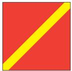
A red panel square with a yellow diagonal stripe signifies that the state of the manoeuvring area is poor and pilots must exercise special care when landing.
