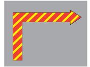
A red and yellow striped arrow placed along the whole of two adjacent sides of the signals area and pointing in a clockwise direction signifies that a right hand circuit is in force.
