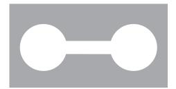
A white dumb-bell signifies that movements of aeroplanes and gliders on the ground shall be confined to paved, metalled or similar hard surfaces.
