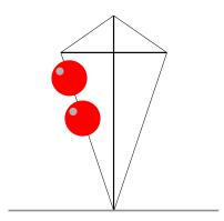
Two red balls disposed one above the other, and suspended from a mast, signify that glider flying is in progress at the aerodrome.
