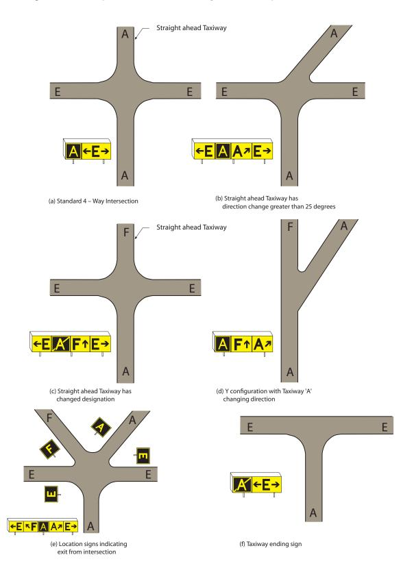
**Figure 3.5** Examples of use of Runway Location Signs and Signs at Runway Taxi-Holding Positions Serving more than one Runway
